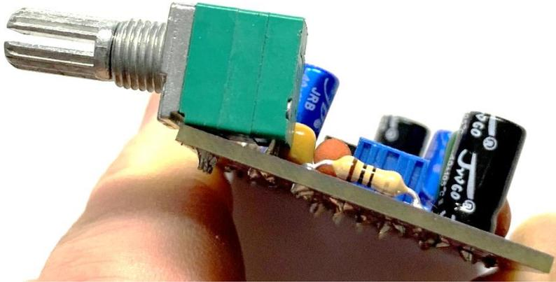
Now refer back to note at the start of the build instructions about snapping off the tag and fitting the control so the back pins JUST are flush with the board, the control needs to be installed at angle to compensate for the slope of the case front.
