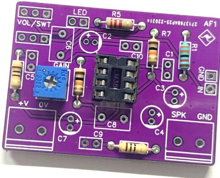
Resistors can be fitted either way round but you must make sure you fit the correct value resistor in the correct place. Resistors have colour bands on them that tell us their value. I have supplied a colour resistor chart that should help you check the value of the resistors. I tend to use a test meter to check any resistors I fit.
