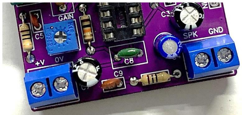
Fit and solder these in place. Now a confession, when I designed this board it would have been better if I gave you a larger soldering pad for each of these terminals and I will on the next batch of boards but just make sure you solder the pins of the blocks well.
