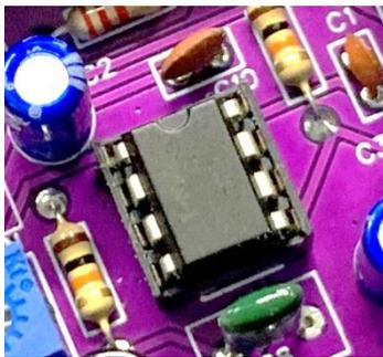
Now before we put the board in place you can fit the IC to the board. The chip has a small notch on one short edge. Make sure this notch is nearest to C10 and C2 on the board.
