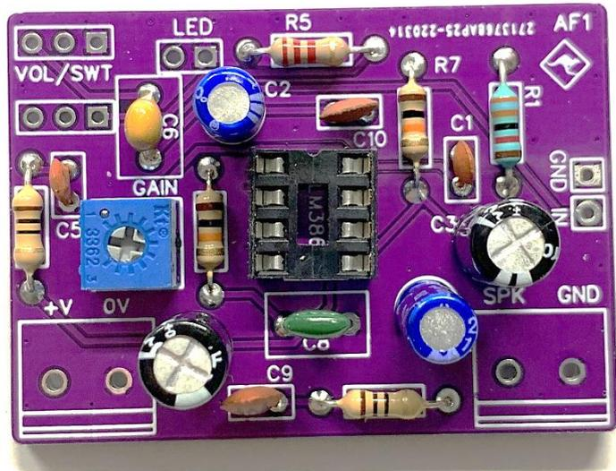
Fit C1 and C5 both of these are 10nF disk type capacitors. They will be marked 103 on one side of the disk. These can be fitted either way round.
