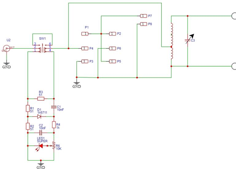
The EFHW uses a resistive SWR bridge with adjustable sensitivity, works well from a few 100mW up to the power limit of the ATU, I recommend keeping the power to QRP levels maybe a little more when matched. Please ignore resistor ref numbers shown on the circuit as they changed on the new PCB.
