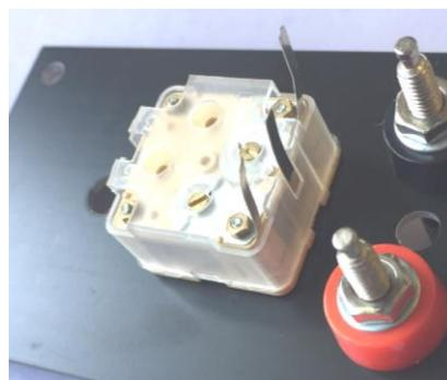
Now Remove the **TOP** nut and washers from the switch (not the bottom nut), drop the LED into the PCB just in front of the switch. Make sure that the long leg of the LED is nearest to the switch (the round hole). DO NOT Solder it yet!
