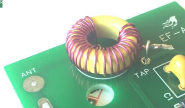
Now I strongly recommend that you use a meter and check for continuity between the ends of the coil. The best place to check this is on the two larger pads marked ANT and CP.
