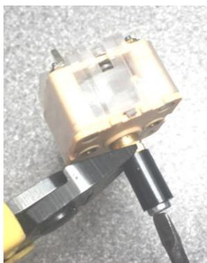
We have now to fit the capacitor to the front panel. First fit the shaft extender, it's a black 10mm long plastic shaft that is secured by a 2.5mm x 12mm screw, be careful here, you can damage the internals of the capacitor by applying too much direct force. Hold the small brass shaft with a pair of cutters while tightening the screw, this keeps any force off the internal parts.
