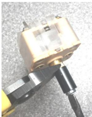
We have now to fit the capacitor to the front panel. First fit the shaft extender, it's a black 10mm long plastic shaft that is secured by a 2.5mm x 12mm screw, be careful here, you can damage the internals of the capacitor by applying too much direct force. Hold the small brass shaft with a pair of cutters while tightening the screw, this keeps any force of the internal parts.
