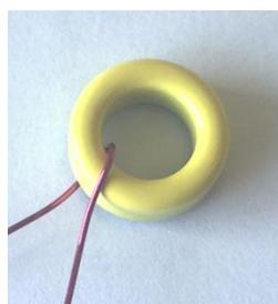
Start with passing the wire through the core as shown. Now wind 3 turns around the core, each time the wire passes through the core it counts as a turn. The short end of the wire should be down at 6 O'clock position as we
