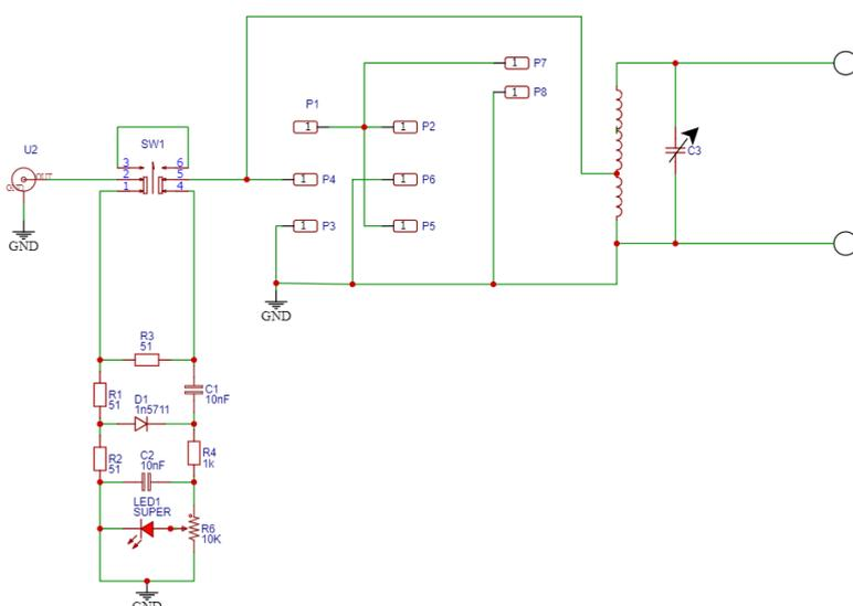
The EFHW uses a resistive SWR bridge with adjustable sensitivity, works well from a few 100mW up to the power limit of the ATU, I recommend keeping the power to QRP levels maybe a little more when matched.
