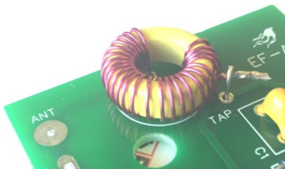
Now I strongly recommend that you use a meter and check for continuity between the ends of the coil. The best place to check this is on the two larger pads marked ANT and CP.
