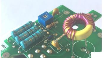
Ok you kept the offcuts from the resistors didn't you? I hope so. Use one of these offcuts to connect the PCB to the coils tap, I make a little walking stick hook on one end that goes over the loop and drop it through though the board and the 'hook' over the tap, solder when done (both at the loop and under the board) This core as two long ends and a tap.
