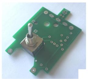
1) Fit the switch first, the switch must sit on the side of the PCB that shows the silk screen picture of the switch and you will see 'SWT' near one edge of the board, make sure that you push the pins through the board and that the switch sits straight and flush.
