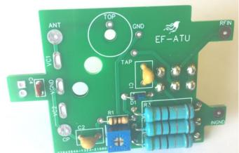
so in a worst case scenario with a short circuit on the output the three will share the full amount of RF power, since we are only using QRP that would be a rated power of 6 Watts but of course we will be only applying power to the tuning bridge for a short time and we hope we will not have a short circuit on the output so these two watt resistors are suitable for our needs. (Also keep the off cuts for now!)
