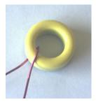
Start with passing the wire through the core as shown. Now wind 3 turns around the core, each time the wire passes through the core it counts as a turn. The short end of the wire should be down at 6 O'clock position as we start winding up towards in the 9 O'clock direction
