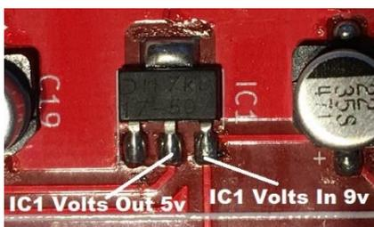
**Note:** PICTURE OF IC1 SHOWING INPUT/OUTPUT PINS TO TEST
