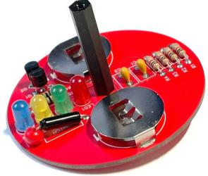
Now fit the batteries, on one side of each battery you will see a '+' sign and some writing. This side of the battery must be on the top as you slide them into the holders.
