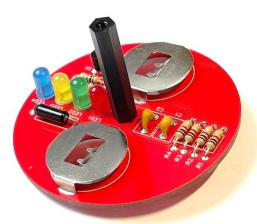
This kit uses a number of common parts such as Resistors, capacitors, LED's and transistor's. The typical type of parts you will find in just about all projects!
