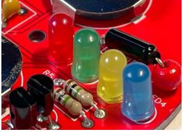
Now we can fit the Switch. The switch is an interesting thing. It looks like big black resistor but in fact it's made up from a metal tube with a ball bearing inside.
