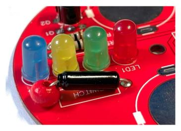
The one problem with such a simple switch is that it can turn on even if the board is just sat on a flat surface, to make sure the spinner only turns on when we spin it we need to fit the switch slightly higher on one side than the other to keep the ball bearing at the bottom of the tube when we are not spinning the disk.
