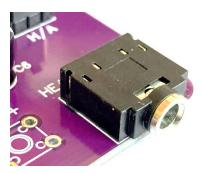
Now we need to fit the 3.5mm stereo headphone socket, this should be fitted so it flush to the board. When fitted trim the leads on the back of the board as flush as you can. One of the stick-on feet will be placed under this part of the PCB later.
