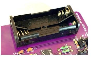
**tape touches the PCB so take care**, when in place solder the two legs. Now put the four stick on feet on the bottom of the board, one in each corner, when you stick them in the front corners you will have to cut any soldered connections nice and flush with the board.
