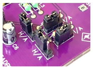
jumpers onto the blocks on the 'H' side (as the picture here)
