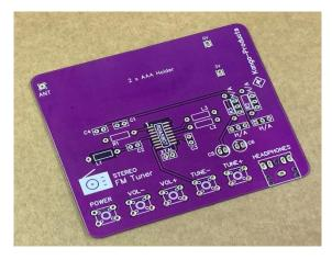
All the locations for parts are screen printed on the PCB so make sure you double check the right part is fitted in the right place!
