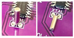
carefully fold the crystal over as in the second picture here. Make sure the legs are NOT shorting out on each other. Double check that you have also not shorted out the two pins on the solder side of the board, the solder pads are very close to each other. Tick of when done these steps
