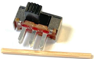
Put the switch on the PCB and insert the stick though the legs as shown here.
