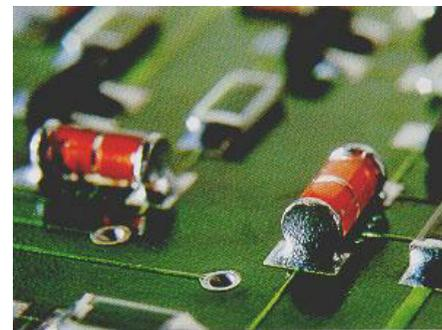
Heat the currently unsoldered end of the component and the adjacent pad with the soldering iron, and carefully wipe on a small amount of solder. You want a small fillet as shown in the illustration, not a large glob of solder.
