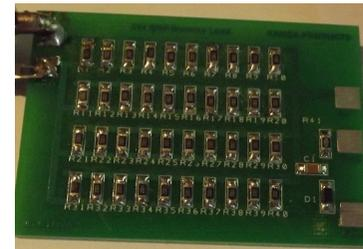
A dummy load is a resistor equal to the output impedance of a transmitter. It is used to convert the output power to heat instead of feeding it to the antenna.
