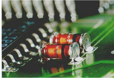
After the joints have cooled, inspect them carefully to make sure that they are solid and make contact with the board. If you have any doubt about the quality of the connections as in the picture not enough solder, apply more flux and reflow the joints until you are satisfied.
