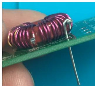
These hooks are fed through the board to connect the coil taps to the PCB.
