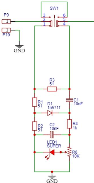
This section can be switched IN or OUT by a two way toggle switch, when in circuit the bridge will light the LED if the antenna is presenting an impedance higher (or Lower) than 50 ohms, if the impedance is matched the LED will go out. Depending on the power level in use the LED can be either too bright and doesn't go out when matched or too dim and hard to see. This circuit has an adjustable sensitive trimmer and it is best to adjust this to suit your most likely used power level.
