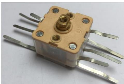
On one side of the capacitor there are 4 pins, the other side has 5. Make sure you identify each side
