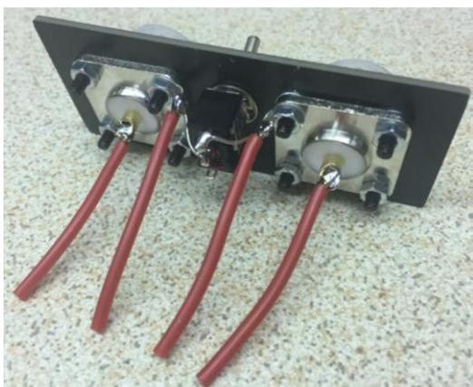
Now fit the links to the back panel, I have provided some silicone coated wire for this, it's very flexible.
