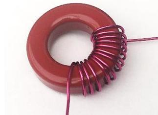
Continue to wind the wire for a total of 13 turns as in the picture on the right.
