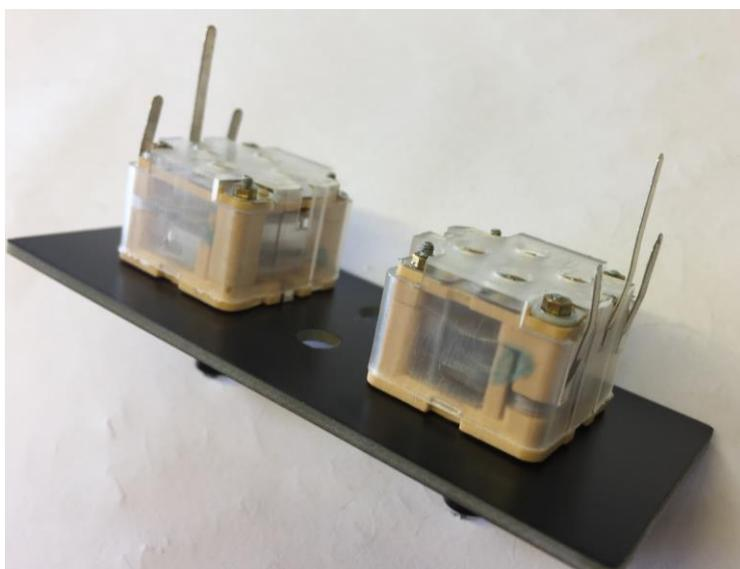
Fold back the three remaining terminals from each capacitor as shown in this picture.
