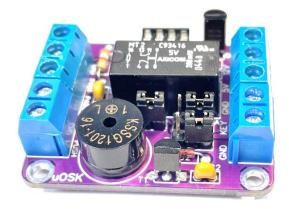
Next fit the sounder, this is for side tone. This if you look on the top of will have a '+' mark on one side. This should be near the relay on the PCB. (See photo here).
