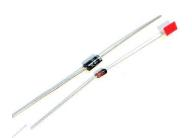
Now we can fit the two diodes, D1 first, this is a 1 amp diode (something like a 1N4001 to 1N4007) and is much bigger
