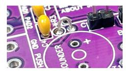
• We have a position marked on the board R3. This is to allow you to fit a resistor if you wish to lower the sidetone volume, try around 100 ohms (Customer supplied). Most customers are happy with the level as designed and so just fit a link from a resistor offcut in this location.
