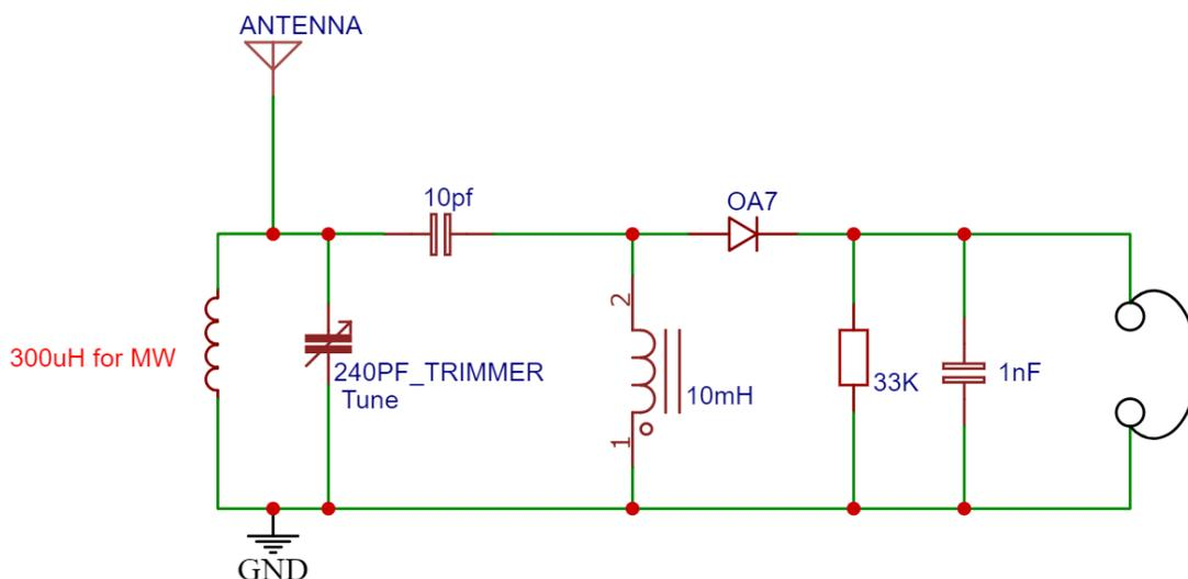
We have now altered the circuit more to allow the antenna to be inductively coupled to the tuning coil to improve the performance from the circuit above.
