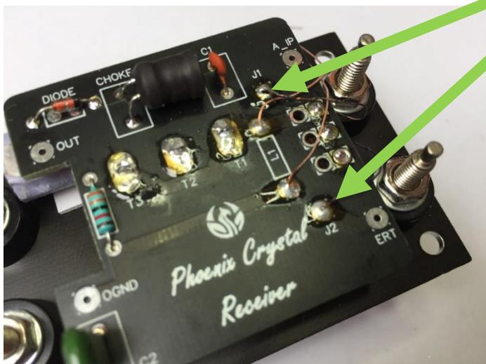
In the picture above it can be hard to see these black wires so I have shown the positions that they must be soldered to.
