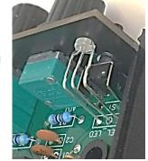
When the board and front panel are fixed together put the LED into the PCB and then push the LED though it's hole on the front panel. Now we can solder the LED in place
