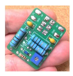
There are many factors that should be considered when measuring SWR as it's not just a resistive load, but in practice this type of circuit does the job fine and 1000's of people use this type of bridge with good success.
