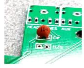
All the capacitors can be fitted either way round but I suggest fitting them so that the value is shown all on the same side. This makes it easier for fault finding should you need to.
