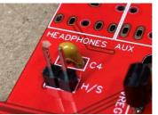
There are 6 pairs of header pins for you to fit, don't forget the one just behind the headphone socket.
