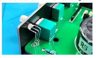
**Before** fitting the switch use the four small PCB mounting screws to fit the PCB into the case, check the positioning of the board from the rear to get the jack sockets lined up with the rear panel holes.
