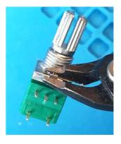
Now fit all three controls, the volume control also has a built in on/off switch and will only fit in one place, either of the other two can be used for the speed and gap controls (they are the same value)
