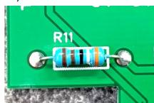
Be careful, these can be mistaken for the 39 Ohm resistor, the first different you will see if you look at both is that these resistors have 5 bands , the 39 Ohm resistor has only 4 bands.
