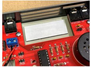
Now you will also have a length of foam tape,. Cut the length to fit the cut-out in the PCB for the battery and stick the foam pad to the bottom of the case.
