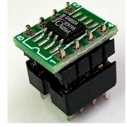
outline of a standard chip with a notch at one end, this end should be nearest to the notch on the socket.
