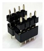
Now drop the adapter board on top of the pins. Take care and solder each pin to the adapter board. Now you can treat the assembly the same as a standard chip. Make sure that the 'chip' is plugged into the socket the right way round, if you look at the top of the chips board you will see the printed
