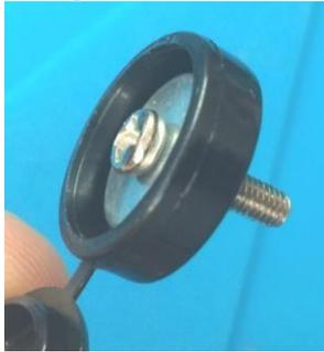
Find the flange, the 3mm white spacer, steel washer, the Key top panel and a M3 steel nut.
