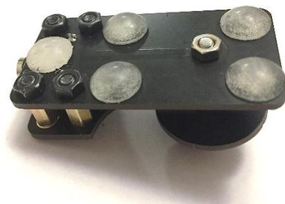
That's it the key is built and ready to test, connect a lead from the keys socket to the radio or oscillator and tap away.
