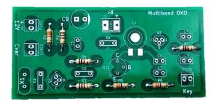
Now double check all are fitted correctly and trim the leads flush to the board.
