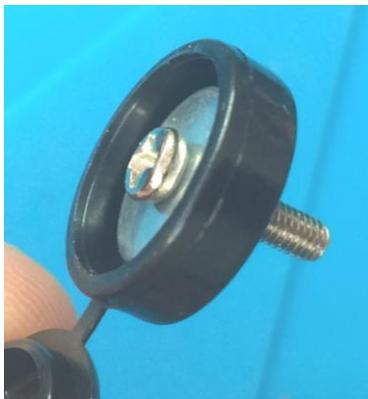
Find the flange, the 3mm white space, one small steel washer, the Key top panel and a M3 steel nut.
