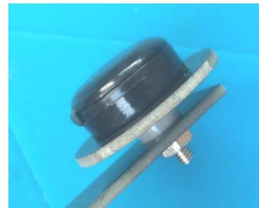
screw and nut securing the knob and flange. This screw also serves as the top 'contact' point for the key. You may need to remove or add a washer as detailed here to set the gap to your liking, this is a good starting point for most people.
