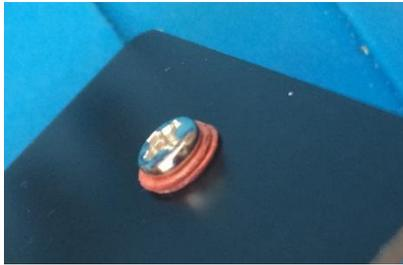
Step One:- Fit the bottom contact screw. Find the 6mm Screw (The shortest in the kit, note yours will maybe a flat slot head) and BEFORE putting it on the bottom board put two of the small Steel washers onto the screw (you may be removing one or adding one later to adjust the gap to your liking).
