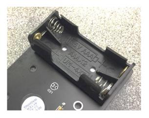
battery holder down to an acceptable size, you can re-trim these if you feel the need but they are very hard pins and I recommend using old cutters as they can damage the low cost cutters blades and also wear eye protection if you can, these legs can fly off at speed when cut.
