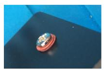
Step One:- Fit the bottom contact screw. Find the 6mm Screw (The shortest in the kit, note yours will maybe a flat slot head) and BEFORE putting it on the bottom board put two of the small Steel washers onto the screw (you may be removing one or adding one later to adjust the gap to your liking). Put the screw through the single hole at the one end of the base panel. The screw head is the bottom key
