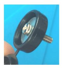
Find the flange, the 3mm white spacer, one small steel washer, the key top panel and a M3 steel nut.
