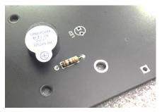
Next fit the 1K resistor. It is the only resistor in the kit, it can be fitted either way around.
