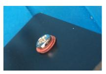
Step One:- Fit the bottom contact screw. Find the 6mm Screw (The shortest in the kit, note yours will maybe a flat slot head) and BEFORE putting it on the bottom board put three of the small Steel washers onto the screw (you may be removing one or adding one later to adjust the gap to your liking). Put the screw through the single hole at the one end of the base panel. The screw head is the bottom
