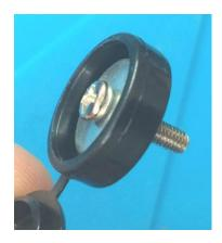
Find the flange, the 3mm white spacer, the key top panel and a M3 steel nut.
