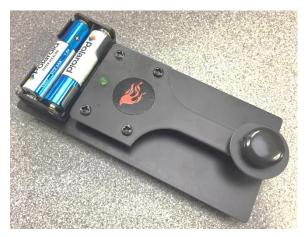
The sticker has not just been included for cosmetic reasons. Try this, hold the key down. Now place your finger tip over the hole in the top of the key panel, you will note that the tone changes. I feel it sounds better with the hole covered, the back pressure blocking the hole just above the sounder changes the pitch and tone qualities. If you agree then place the sticker over the hole.
