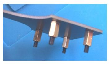
Find the four Brass 10mm spacers and the four black 16mm screws. Pass the screws through the top of the key panel and secure the spacers as shown.
