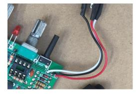
Next to the mode switch you will see three holes marked Key. This is the connection point for the key, the square pad is the GND or common pin for the key and the other two are the left and right paddle connection points.
