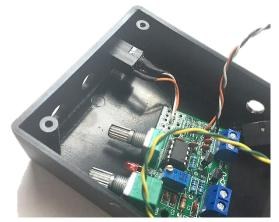
Once you have fitted the key jack then push the PCB in place making sure the LED (and push switch) is seated in their holes, use the washers and nuts provide to secure the board. You will have a little 'jiggle room' to make sure the switch is not trapped against the edge of its hole.
