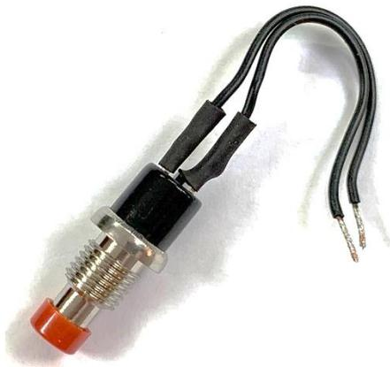
With the kit you will find a short length of wire and some heat shrink. Solder the wire to the two pins of the push button and use the heatshrink to make things nice and tidy, cut the leads to about 50mm.
