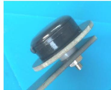
serves as the top 'contact' point for the key. At some stage in the future you may decide to remove the red washer (or add another) as this inconjunction with the red washers on the bottom contact control the key gap.
