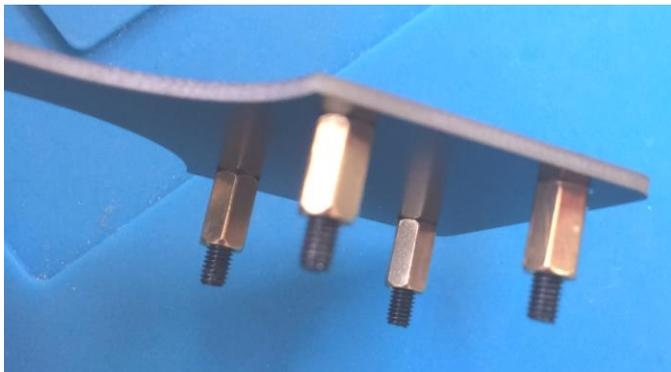
Find the four Brass 8mm spacers and the four black 14mm screws. Pass the screws through the top of the key panel and secure the spacers as shown.
