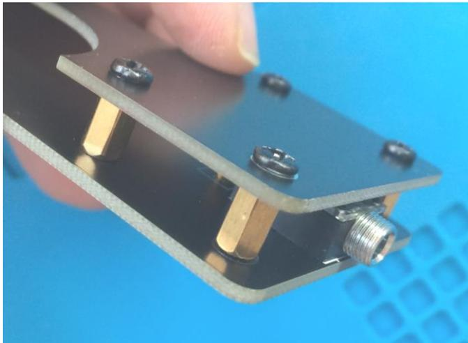
Now drop the top panel onto the base, the black screws should line up with the four fixing holes in the base. Use the four black M3 nuts to attach the two halves. You have two fibre washers left over, these can be used to adjust the gap height. You could easily lose these so I suggest put one under each of
