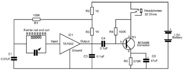
The Ferrite rod and coil can be a old one from a broken radio or approx. 60 turns of thin enameled wire on a 3-4 inch ferrite rod.
