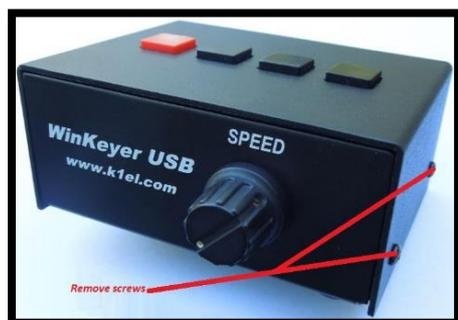
Remove the 4 x screws that hold the case together. Two (2) either side. Now carefully lift the top off, from the front and then slide toward you. Taking care that the sockets on the rear clear the holes before lifting off altogether, and without straining the cables.
