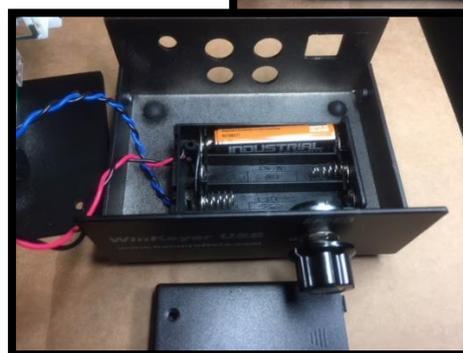
The batteries should last approx. 1 year with normal use. Once the batteries are fitted you will hear “**R**” in Morse, replace the battery cover and gently replace the Keyer Top, inserting the Rear sockets first (reverse of opening the case). Replace the screws, and you are now ready to test and use your WKUSB Keyer.
