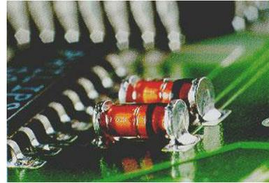
After the joints have cooled, inspect them carefully to make sure that they are solid and make contact with the board. If you have any doubt about the quality of the connections as in the picture not enough solder, apply more flux and reflow the joints until you are satisfied.
