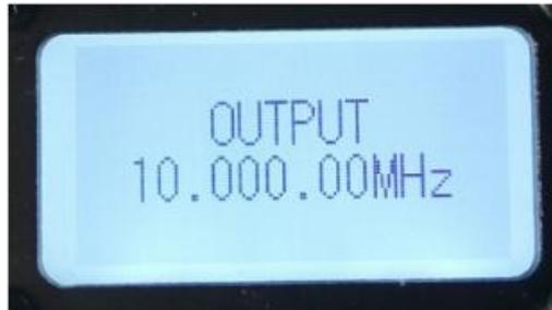
At this time, use the frequency counter to detect the frequency of the TEST point on the PCB board (near the power socket), turn the large knob to adjust the frequency to the frequency counter display 10.000.00MHz, then press the M/V/SAV button to exit.
