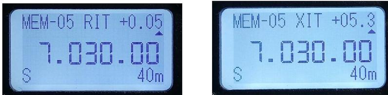
tap of this button will enter or exit the Receive Fine Tune and Transmit Fine Tune (RIT and XIT) functions. At this time, the RIT or XIT and the fine adjustment of the fine adjustment are displayed on the upper right of the LCD screen. **Pressing the tuning large knob after entering the fine tuning state will switch between receiving fine tuning RIT and transmitting fine tuning XIT.**
