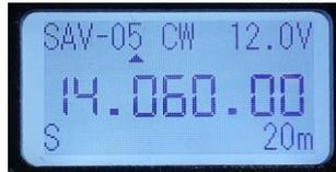
Press the M/V/SAV button for more than 2 seconds to store the current frequency and operating mode to the current memory location. The Sav-\*\* text will be displayed in the upper left corner of the LCD screen. **Each time when turned on, it will enter the frequency and working mode of the last time it was stored**
