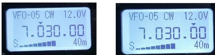
Tap the large knob step frequency to switch between 10Hz, 100Hz, 1KHz and 100KHz. When the step frequency is changed, there is a small triangle mark above the corresponding frequency display position of the LCD screen. If you press the large knob while in the MEM state, it will enter the VFO working state.
