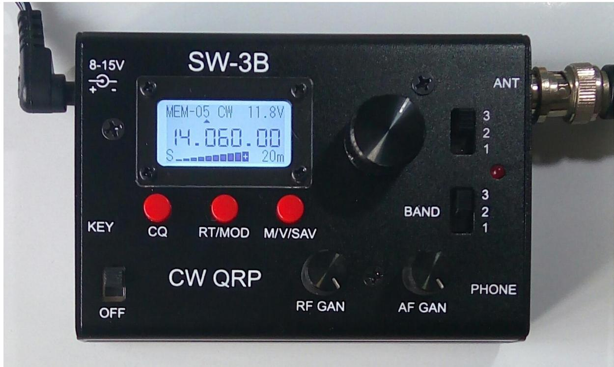
SW-3B is an ultra-small, ultra-lightweight three-band CW QRP transceiver that consumes less than 40mA when receiving. It is ideal for portable use, field day and SOTA.
